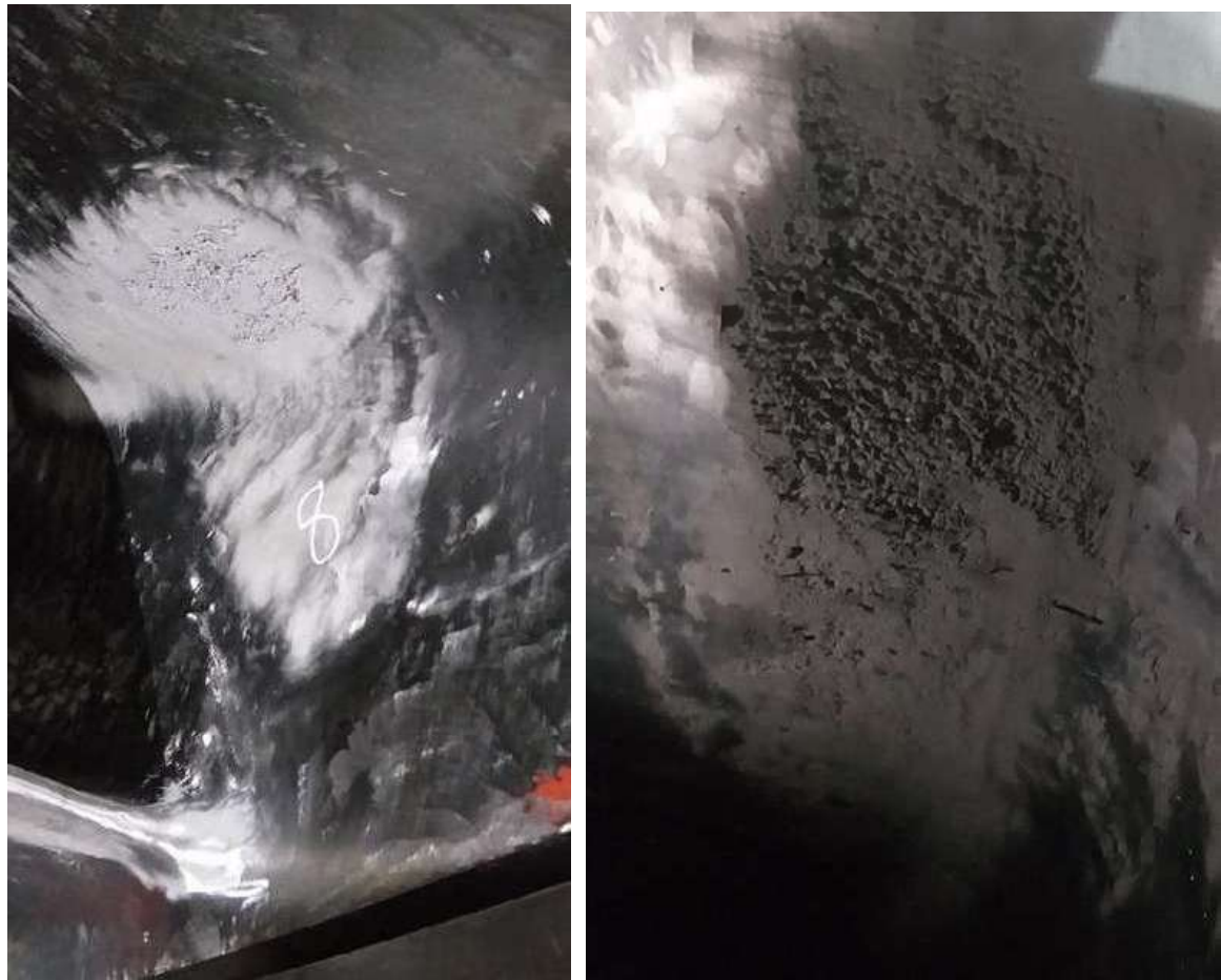
Figure 26: Turbine blade low pressure area cavitation
