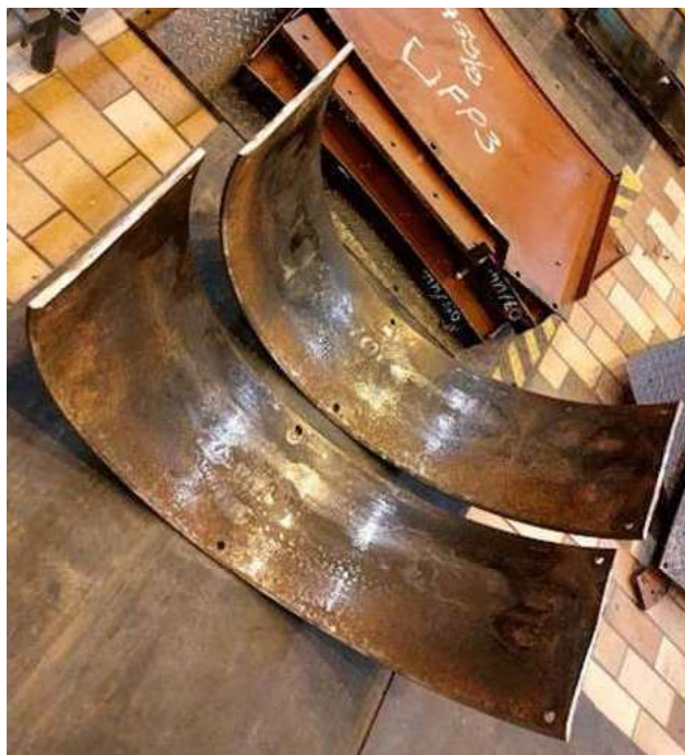
Figure 33: Example of new shaft seal sleeve segments
