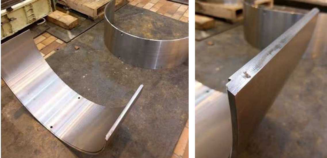
Figure 33: Example of new shaft seal sleeve segments
