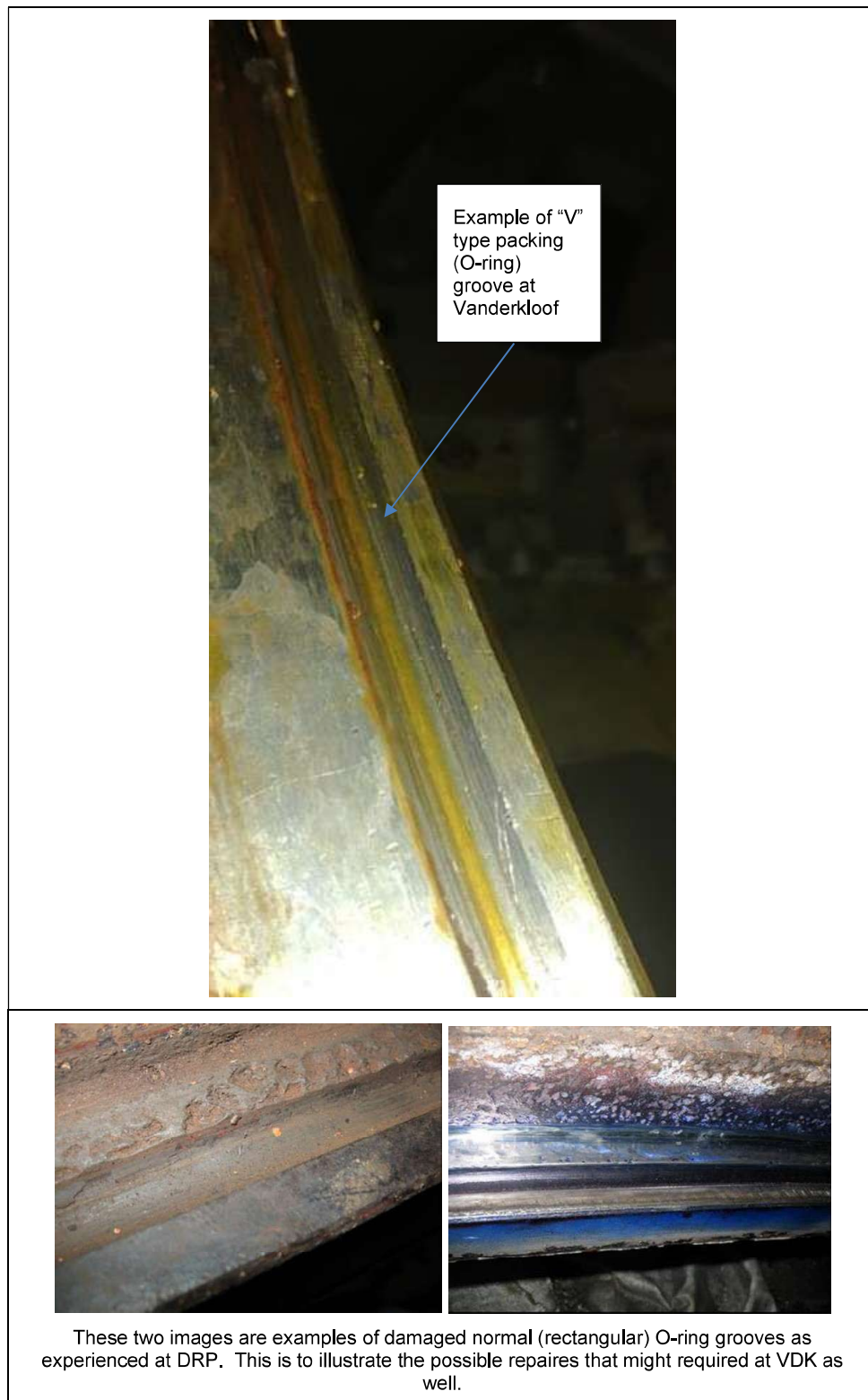
Figure 17: VDK V-type Packing (O-ring) groove
