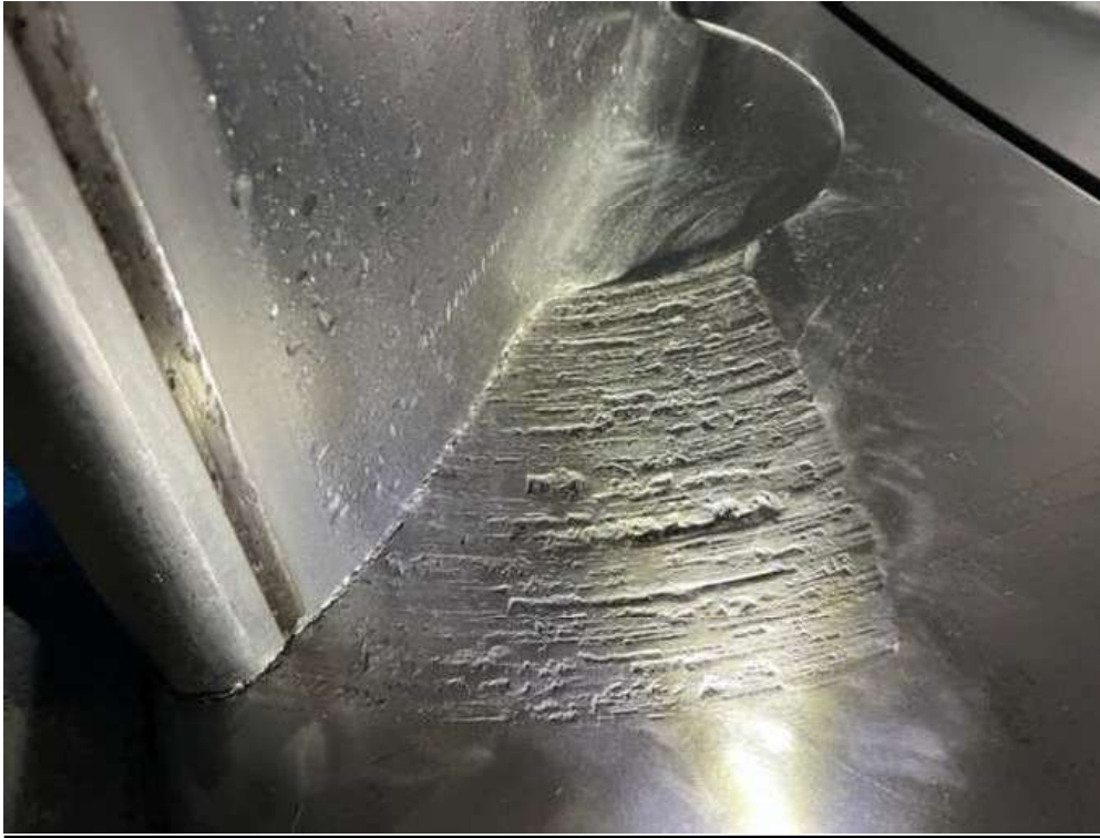
Figure 23: Typical pick-up damage on the guide vane facing plates
